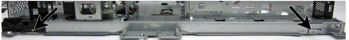
Figure 6-86 Display panel screw locations – 6300 models – CMI panel
